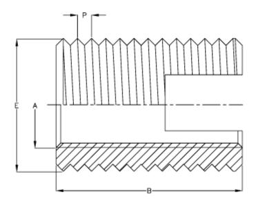
Female thread A = M24 Length B = 30 Male thread E = 30.0 Min hole depth blind hole = 36
